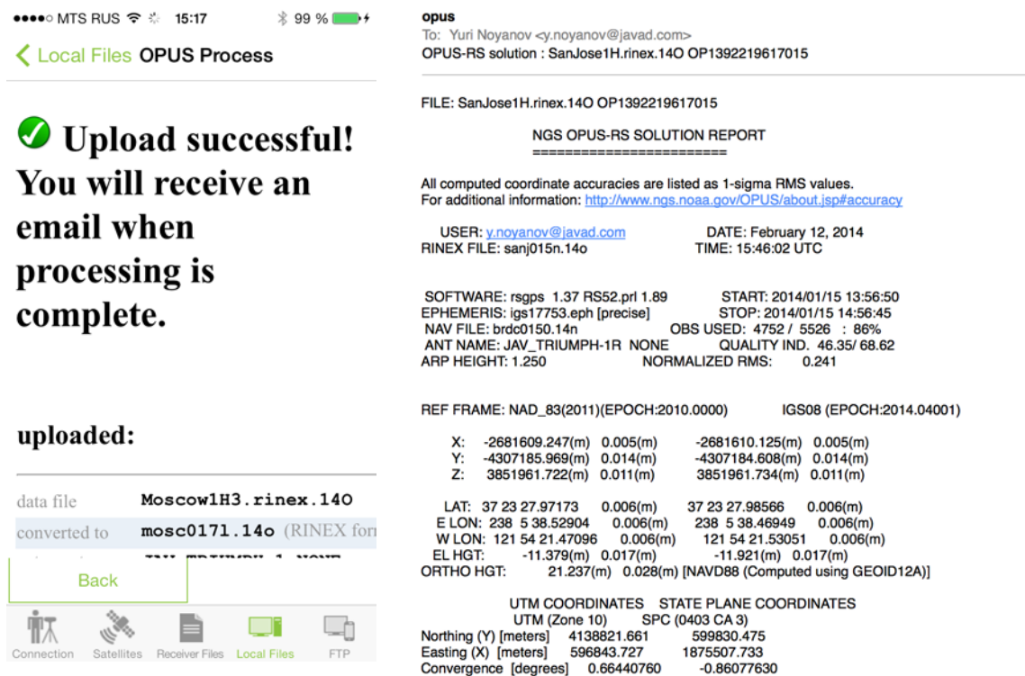
Figure 12. Response from OPUS and OPUS solution report
